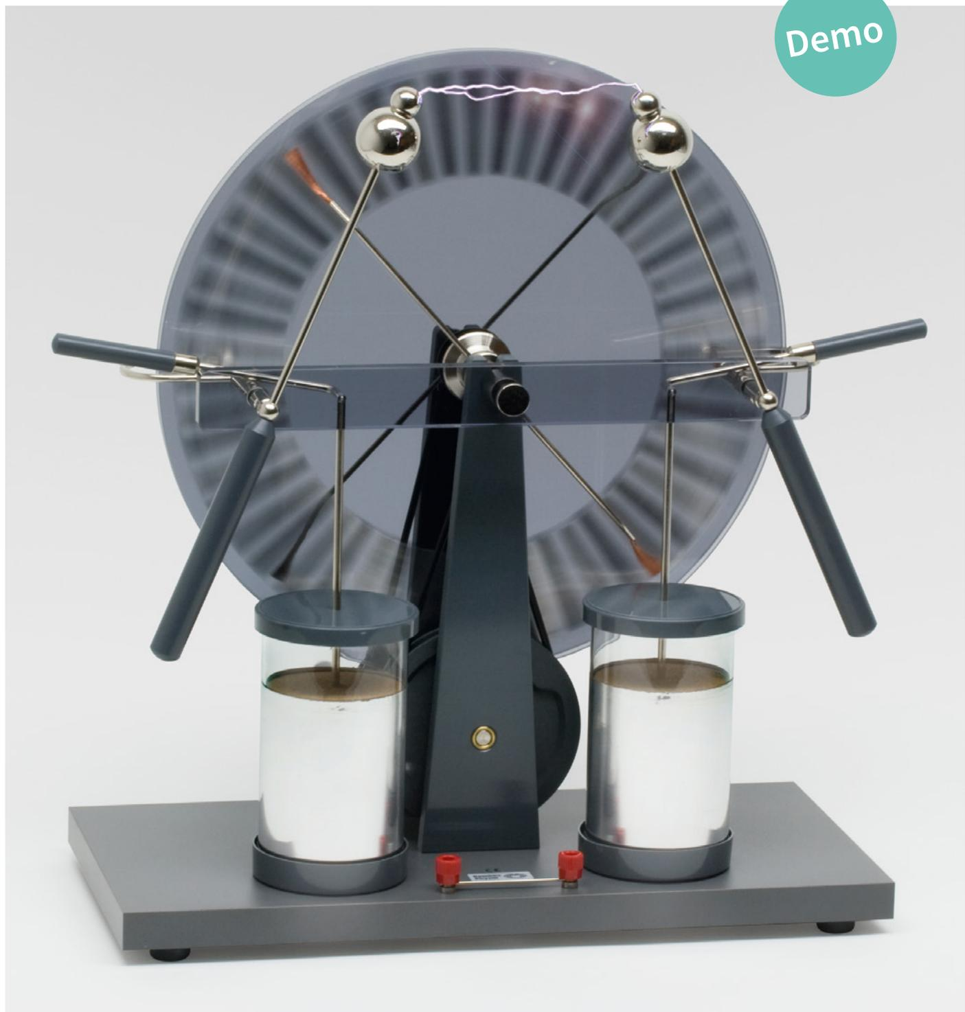
For the continuous production of high electrostatic charges. Mounted on plastic covered wooden base, with crank and belt drive, high insulating perspex discs with metal sectors, two large Leiden jars and spark gap. Including dust protection cover. CE labelled.
