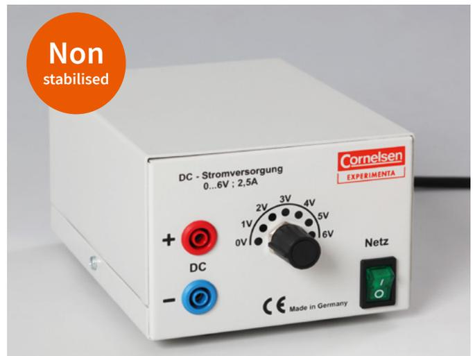
In ventilated steel case, on/off switch with control lamp and mains cable. 4 mm safety output socket terminals for DC. Thermal overload and short circuit protection. CE labelled.
