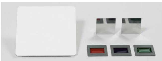
Consisting of two plane metal mirrors on magnetic stand bases, one each foil filter red, blue and green in frame and a 30° inclined screen of white plastic on magnetic base.
