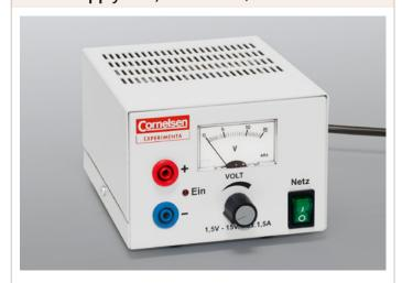
In ventilated sheet steel case with rubber feet, mains connecting cable, coloured, insulated 4 mm safety connecting sockets, on-off switch with built-in control lamp, fused with automatic breaker, activated either thermal or electromagnetic, all outputs galvanic cut from mains. With ground terminal. CE-labelled.
