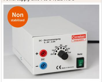
In ventilated steel case, on/off switch with control lamp and mains cable. 4 mm safety output socket terminals for DC. Thermal overload and short circuit protection. CE labelled.
