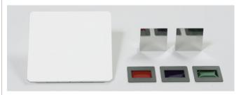
Consting of two plane metal mirrors on magnetic stand bases, one each foil filter red, blue and green in frame and a 30° inclined screen of white plastic on magnetic base.
