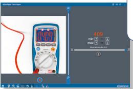
The camera is used to read measurement data, e.g. from digital displays (scales, multimeters), liquid columns (burettes) or needle deflections on dials (hygrometers, ammeters, blood pressure monitors). This data is then available in digital form for further analysis.
