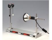
If the elevated tank is connected via the supplied hoses to the solar collector, there will arise a difference in density of the water dependent on the temperature which will cause convection to occur, thus circulating the water.
