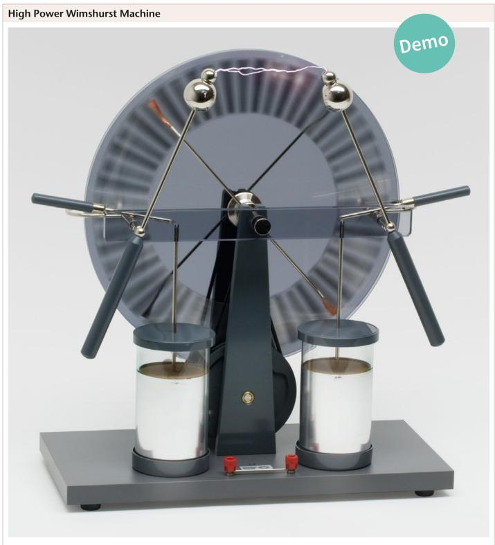
For the continuous production of high electrostatic charges. Mounted on plastic covered wooden base, with crank and belt drive, high insulating perspex discs with metal sectors, two large Leiden jars and spark gap. Including dust protection cover.
