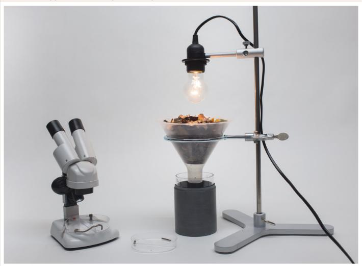
The Berlese apparatus (also known as the Berlese-Tullgren funnel) was developed for the biological investigation of soil samples. It is primarily used to sort out microorganisms (microarthropods) from mulch, leaf litter and pine needle litter for experimental purposes.
