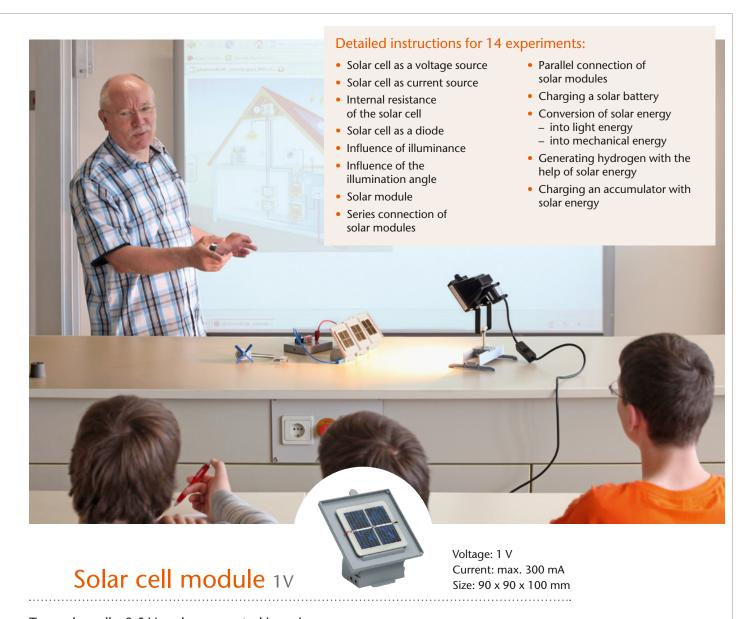
Two solar cells, 0.5 V each, connected in series, mounted on base with hinged panel and 4 mm socket terminals. To increase voltage or current a number of solar cells can be connected in parallel or in series by means of the *Connecting Plugs 54583*.
